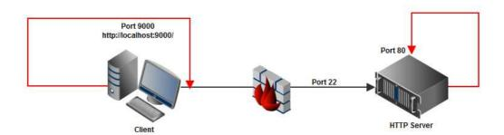
In order to tunnel the HTTP traffic, the SSH client listens on port 9000 on the client. 9000 is an arbitrary port—you can choose any port that is not already taken on the client. When we point our browser at <a href="http://localhost:9000">http://localhost:9000</a>, the traffic is sent through the tunnel, where the SSH server is connected to our web server port listening on port 80.
